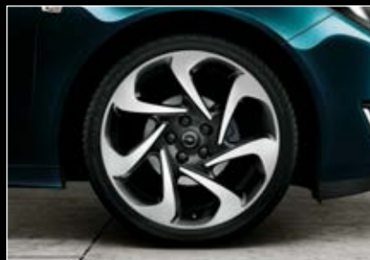
Jante alliage, 8,5 J x 20", 7 branches finition bicolore, pneus 245/35 R 20 (Q7R).
